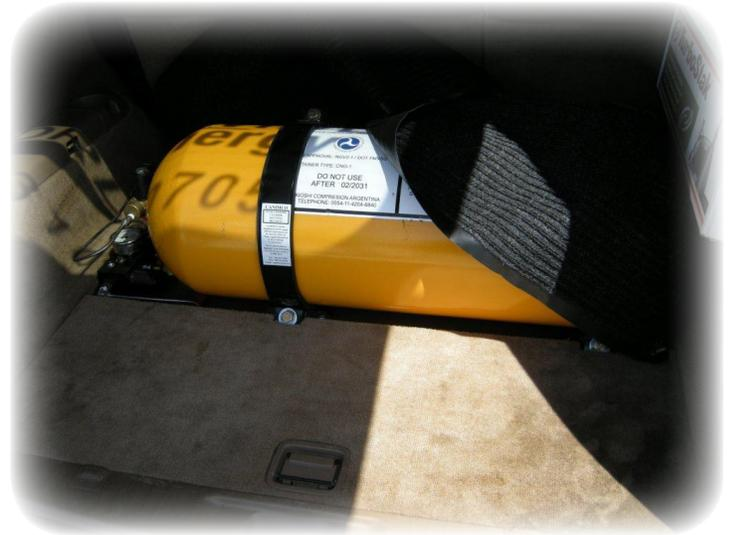
the cargo area of the SUV converted to compressed natural gas. The dump truck on display had a total of three tanks located between the cab and the dump bed. Some of these tanks have up to 3,000 psi. The tanks have a built in pop-off valve for fire or other emergencies. Compressed natural gas is only combustible when the concentration is from four to 14 percent according to Missouri Gas Energy officials. This gas will not concentrate in
