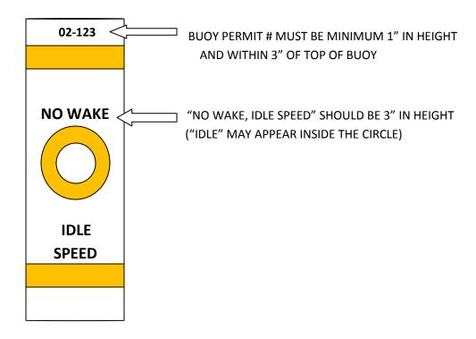
ORANGE REFLECTIVE TAPE SHOULD BE USED AS INDICATED ON THE SAMPLE. LETTERING/NUMBERING SHOULD BE BLACK IN COLOR AND BLOCK STYLE. THE BUOYS MUST BE MAINTAINED IN A LEGIBLE MANNER AND SHOULD EXTEND APPROXIMATELY 36" ABOVE THE WATER.
