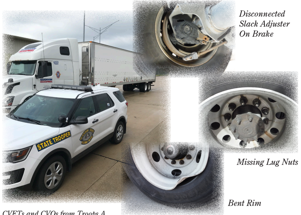
The photos with this story show examples of violations found during the Troop A Truck Check.
